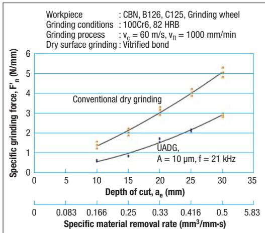
**Fig 10 Specific grinding forces as a function of depth of cut  $a_e$ ,  $v_{ft} = 1000$  mm/min**
