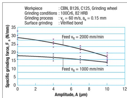
**Fig 3** Specific normal grinding forces as a function of vibration amplitude
