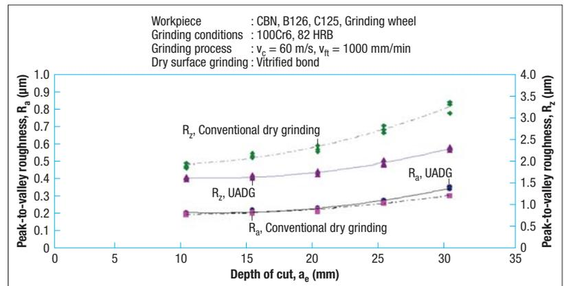
**Fig 12 Surface roughness values  $R_a$  and  $R_z$  as a function of depth of cut  $a_e$ ,  $v_{ft} = 1000$  mm/min (UADG:  $A = 10 \mu\text{m}$ ,  $f = 21$  kHz)**
