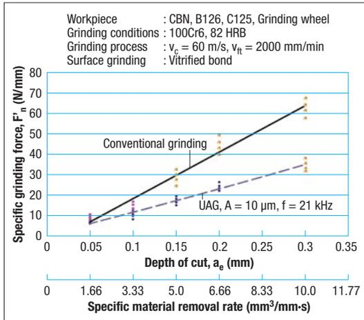
Fig 5 Specific normal grinding forces as a function of depth of cut,  $v_{ft} = 2000$  mm/min (UAG:  $A = 10\mu\text{m}$ ,  $f = 21$  kHz)
