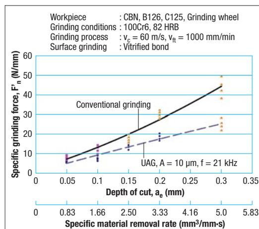
**Fig 4** Specific normal grinding forces as a function of depth of cut  $a_e$ ,  $v_{ft} = 1000$  mm/min (UAG:  $A = 10 \mu\text{m}$ ,  $f = 21$  kHz)
