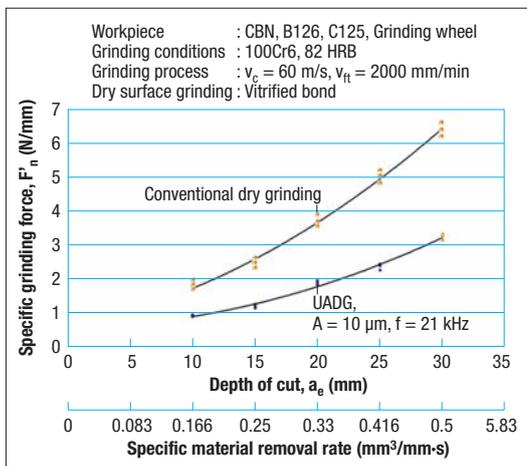
Fig 11 Specific normal grinding forces as a function of depth of cut  $a_e$ ,  $v_{ft} = 2000$  mm/min
