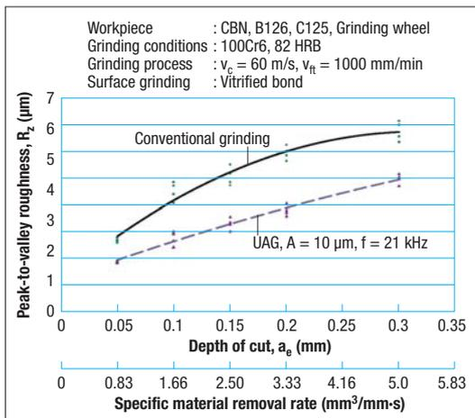
Fig 6 Surface roughness  $R_z$  as a function of depth of cut  $a_e$ ,  $v_{ft} = 1000$  mm/min (UAG:  $A = 10\mu\text{m}$ ,  $f = 21$  kHz)
