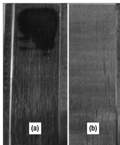
**Fig 2** Burn marks with conventional grinding (a), no thermal damage on the surface ground with UAG (b),
