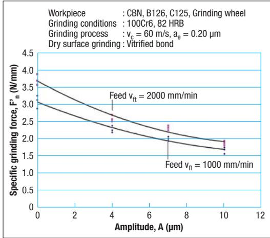
**Fig 9 Specific normal grinding forces as a function of vibration amplitude ( $a_e = 20 \mu\text{m}$ ,  $f = 21$  kHz)**
