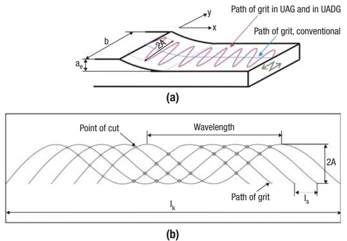
**Fig 14** Path of a cutting edge in ultrasonic-assisted grinding (a) Path of a number of grits that engage the surface of a workpiece simultaneously or one after the other (b)
