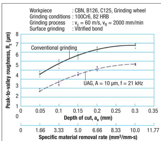
Fig 7 Surface roughness  $R_z$  as a function of depth of cut  $a_e$ ,  $v_{ft} = 2000$  mm/min (UAG:  $A = 10\mu\text{m}$ ,  $f = 21$  kHz)
