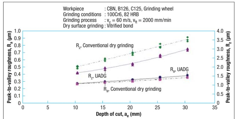
Fig 13 Surface roughness values  $R_a$  and  $R_z$  as a function of depth of cut  $a_e$ ,  $v_{ft} = 2000$  mm/min (UADG:  $A = 10 \mu\text{m}$ ,  $f = 21$  kHz)
