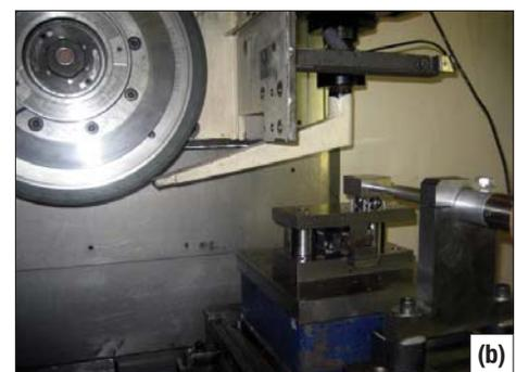
Fig 1 (a) Diagram of the experimental set-up of the vibration chain (b) Test rig for ultrasonic grinding
