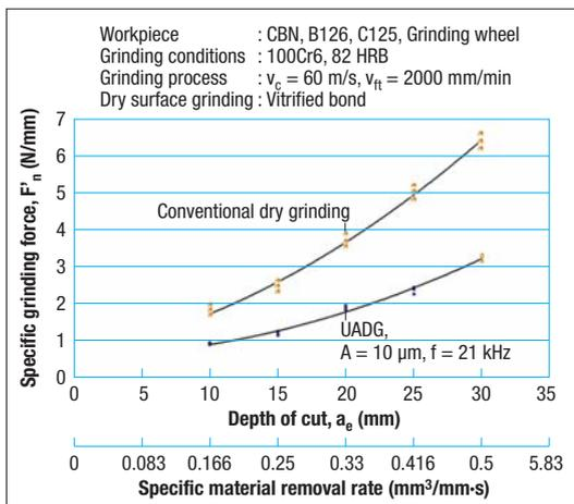
**Fig 11 Specific normal grinding forces as a function of depth of cut  $a_e$ ,  $v_{ft} = 2000$  mm/min**
